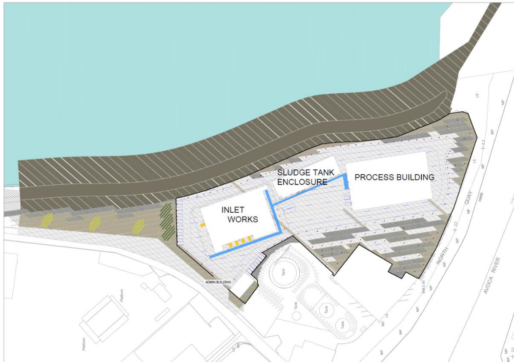
Figure 1: Proposed WwTP site layout
