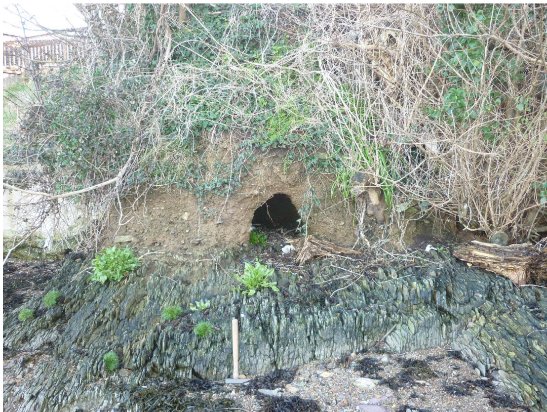
Photo A6/3. Bedrock 1- c.0-5m. Superficial soil deposits resting on strongly cleaved mudstones and heterolithic rocks.
