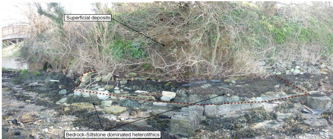
Photo A6/2. Bedrock 1. c.0-20m. Superficial deposits resting on the bedrock which is composed of fine-grained heterolithic rocks with intense fracture cleavage fabric. Red line shows outline of ruined house foundations.
