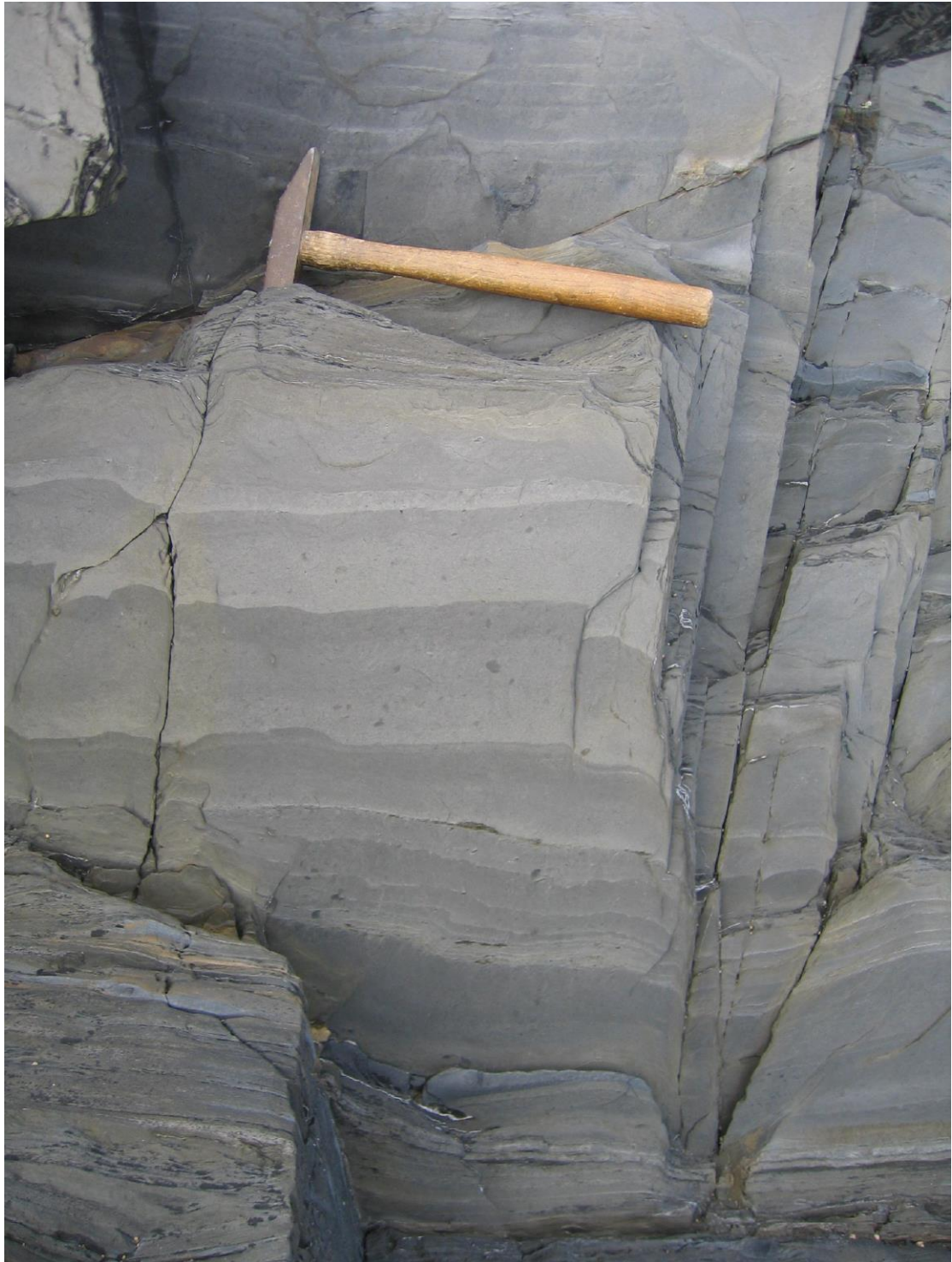
Appendix B23. The Kinsale Formation Castle Slate Member showing jointing, fracturing and lamination.
