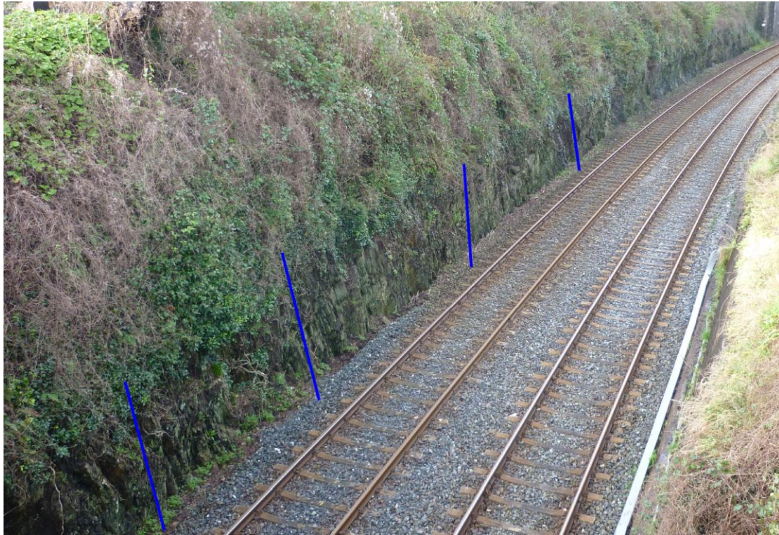
Photo A7/5. This is a view looking northwestwards from Bridge 4 towards Bridge 3. Blue lines show the general development of the cleavage fabric here. The fabric is vertical to sub-vertical and is oriented NE-SW. This is typical of these rocks in the region.
