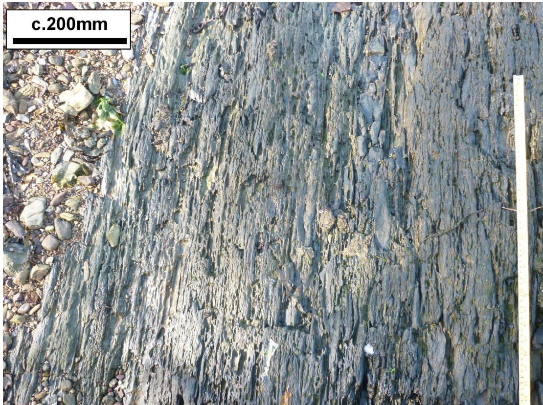
Photo A6/8. Cleaved mudstones and heterolithics at Ringacoltig north. Cleavage planes are parallel to the tape and are closely spaced and inclined steeply to the north (left).
