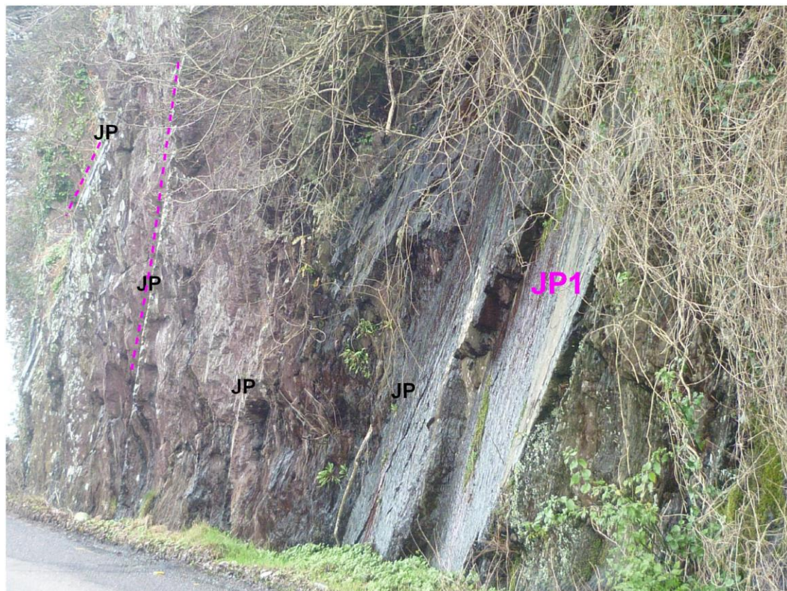
Fig 13.2. Ballytrasna Formation Passage Road, Monkstown showing selected intersecting bedding planes (green lines), joint planes (JP and purple lines) and cleavage planes (red) in purple/red fine-grained sandstones and siltstones. The strike of the joints intersects the strike of the bedding and cleavage at very high angles. The same rock face is shown in both images but viewed from a different angle. JP1 is the same joint plane in both images.
