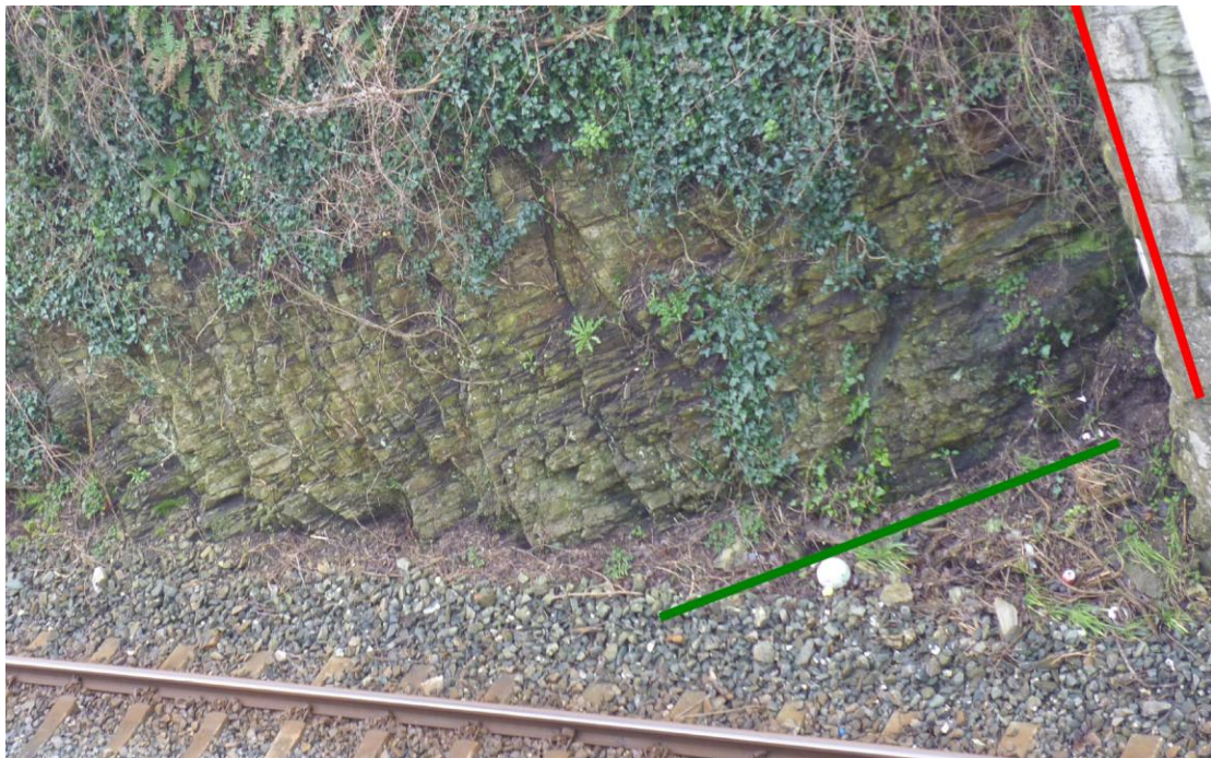
Photo A7/8. Jointing (parallel to the red line) and bedding (parallel to the green line) in the Cuskinny Member on the eastern side of Bridge 4 looking southwards.
