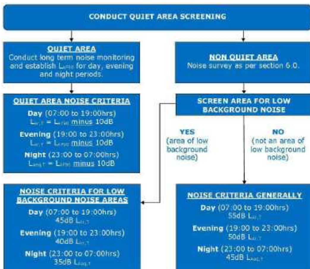
Figure 9-1: Extract from EPA Guidance Note for Noise: Licence Applications, Surveys and Assessments in Relation to Scheduled Activities (NG4) - Steps to be Followed in Order to Derive Appropriate Noise Limit Criteria (Ref. EPA Guidance Note (NG4) (EPA 2016))
