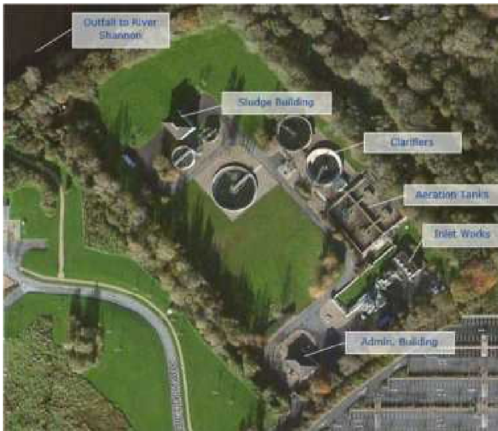
Figure 1-3: Castletroy WwTP Existing Layout
